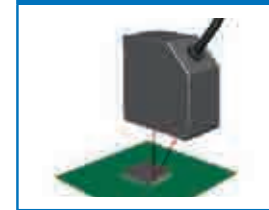
Inspecting for Board Coplanarity
